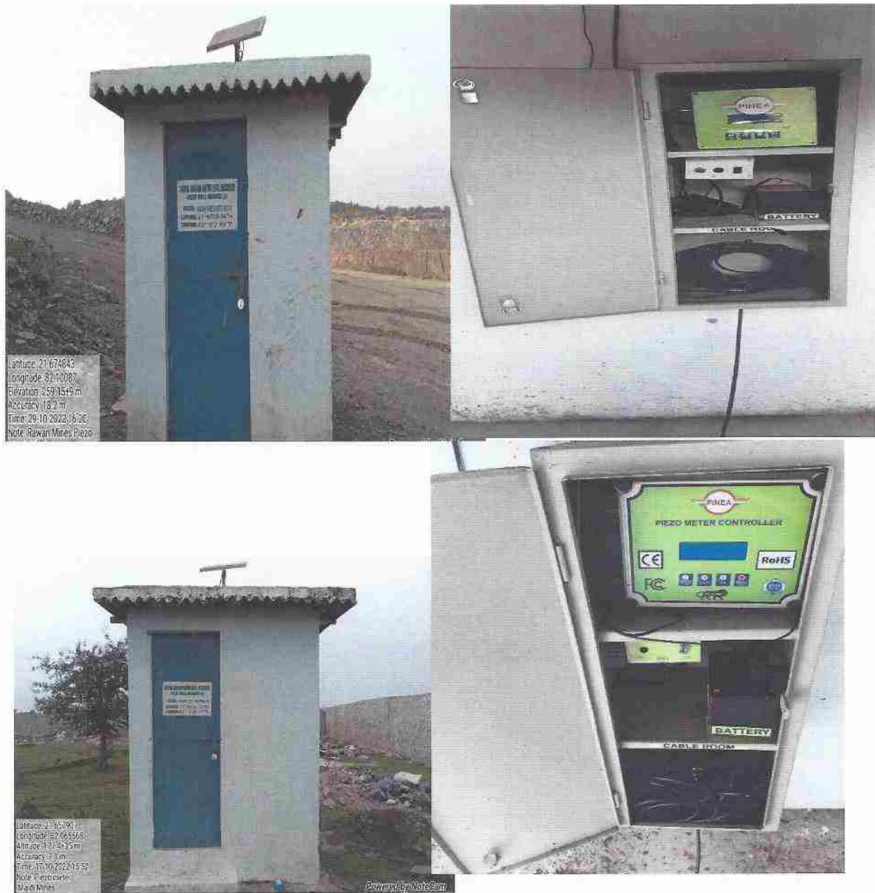
Typical View of online Piezometers installed in Rawan Mine
